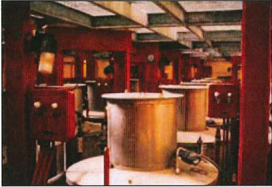
□The Schlumberger Environmental Effects Calibration Facility, Houston, Texas, USA. Over 4000 measurements were made in more than thirty formations of differing lithology and porosity, with different combinations of formation salinities, borehole salinities, and completions to produce the sigma data base.
